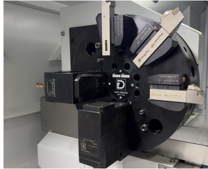
Rear 8-station horizontal-axis electric turret with VDI 30 live tooling (optional) ▶
