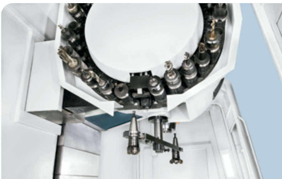
Automatic Tool Changer with 30 tools capacity (ROMI D 800 / D 1000 / D 1250)
